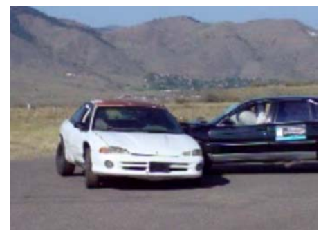
Image of the 90-degree impact of the test vehicle with the target vehicle. Note the inflated driver's airbag.
